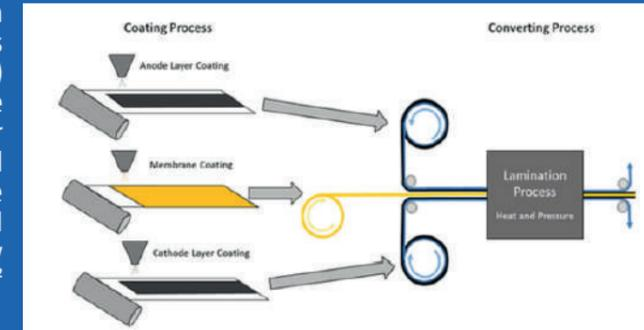
Figure 3. Processes involved in CCM manufacture
