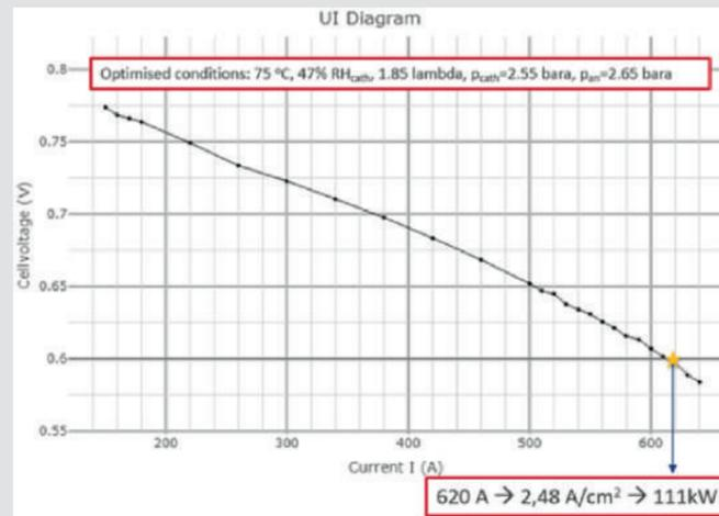
Figure 1. VOLUMETRIQ NM12 stack developed at ElringKlinger.
