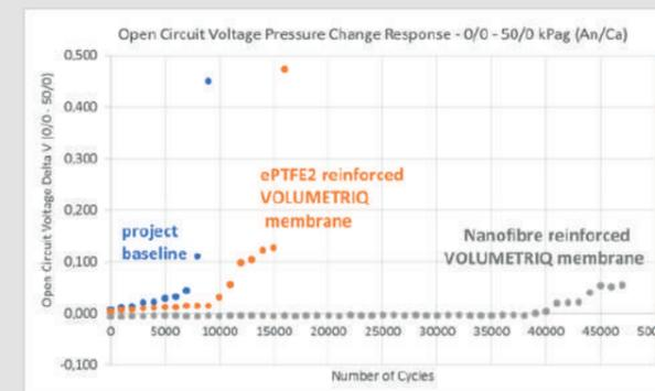
Figure 4. Combined OCV/RH cycling at 90 °C of ePTFE and nanofibre reinforced Aquivion membranes
