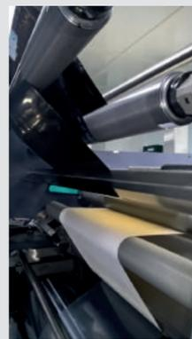
The scaled-up PBI web has also successfully completed the first web handling assessment on a high volume membrane manufacturing coating line at JMFC.
