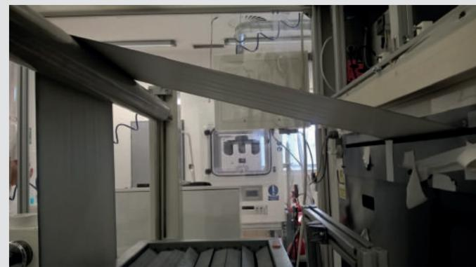
Rolls up to 20 linear metres of electrospun PBI web were successfully scaled-up
